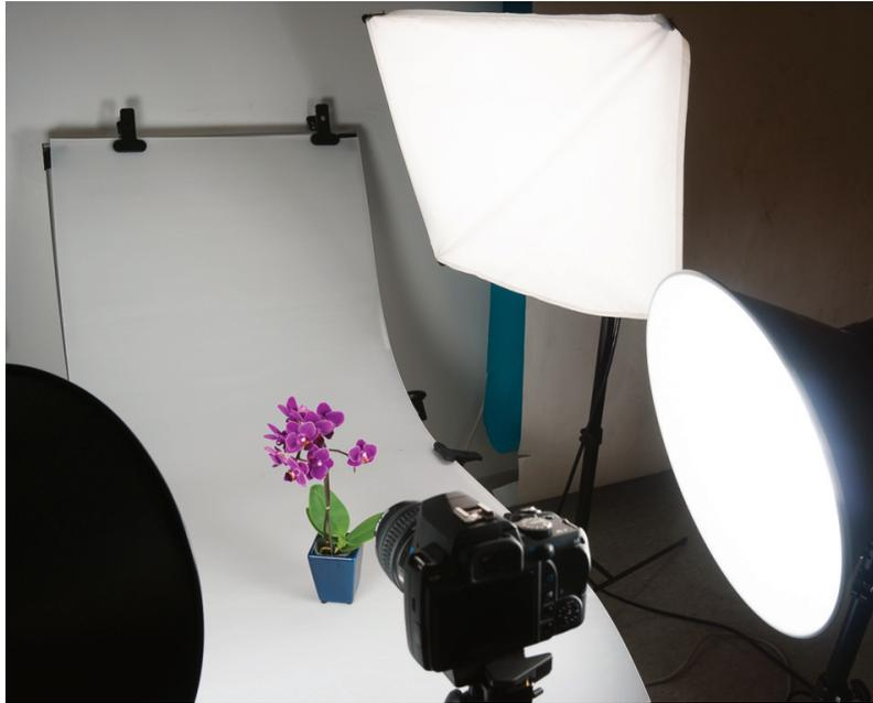
**Figure 14-11.** Studio lights can be equipped with various types of diffusers, including transmissive “soft boxes,” as in the photo, and reflective umbrellas. Photo Richard Adams. Image licensed under CC BY 4.0.
