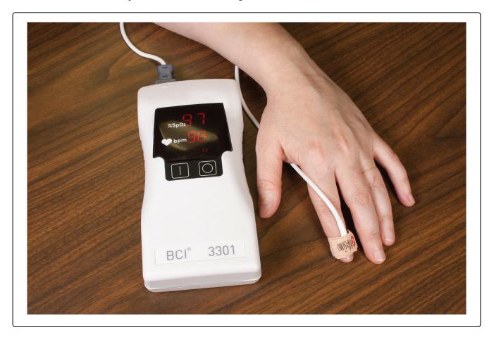
Figure 4.2: Pulse oximeter with sensor taped around finger
